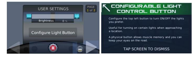
Select the lights you want to turn ON/OFF with each press of the top left button. When your selection is complete touch the check mark gear.
